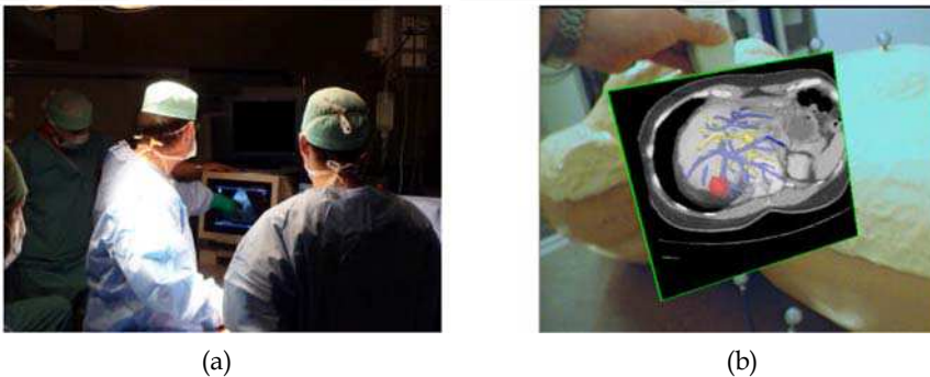
Fig. 3. Overcoming the problem of hand-eye coordination using Augmented Reality (a) Typical examination using sonography. (b) The AR display enables the user to see the data at the same location where his/her hands operate.
